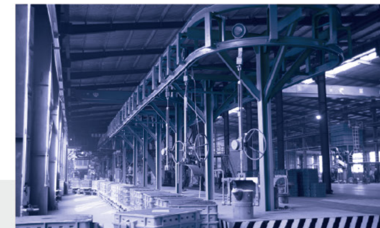
风机配套关键零部件铸造生产线 Casting production line of key parts on blower
